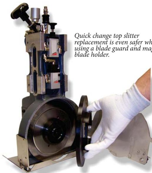
*Quick change top slitter replacement is even safer when using a blade guard and magnetic blade holder.*
