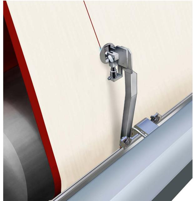
Tail jet cutter is a high-pressure water cutter that cuts the tail and also spreads the sheet after threading. The pressure for the device is provided by a power unit equipped with a backup system.
