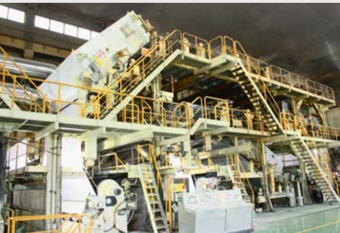
"For this machine Hansol decided also to remove all IRs from the machine and to do all the coating drying with Valmet's OptiDry coat air drying technology."
